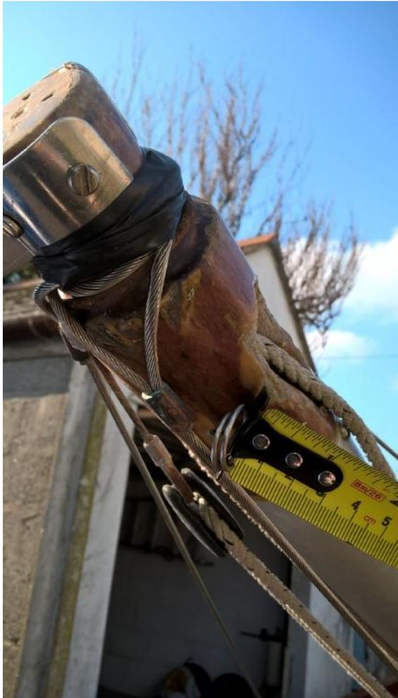
Extend the tape to the transom, pull tight and measure to the horizontal/aft face of the transom. A minimum distance is 355cm (3,550mm). 1 or 2cm more is fine, when you sail you can feel the boat balance and work from that. Don't get hung-up on the numbers, sailing the boat will tell you about your setting;
