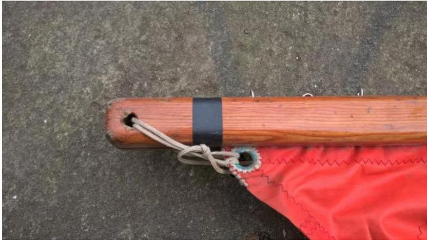
And get the gaff snug and tight up to the mast pulley. The sail is made to give the right shape with a straight mast/gaff. Below the gaff/halliard is too loose (and the boom will be low)
