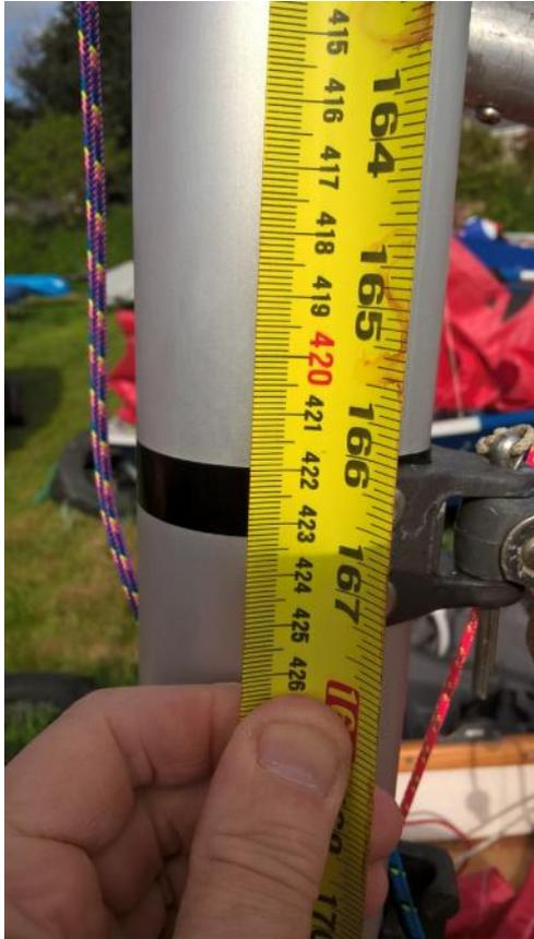
Extend the tape to the transom centre and now measure the length to the rear edge of the transom. For boats with a level transom (wooden and plastic boats like Trident-made) about 5,010mm or 5,020mm will be good. The photo below shows there is more rake – it's a lower number;
