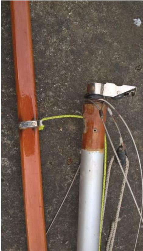
Below the gaff is pulled hard to the mast and gaff band goes into the pulley or sheave;
