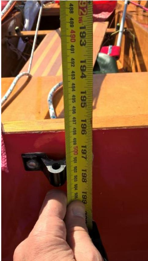
For a curved transom (a Winder made hull) the maximum rake would be 4,990mm. 5,020mm and 5,010mm are good and depends on the adjustability of the shroud plates and shroud lengths.
